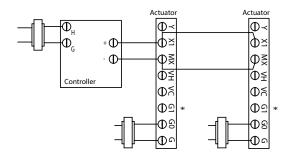
0-10/2-10Vdc Proportional Multiple Actuators powered from separate sources.
