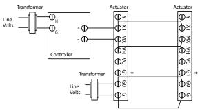
0-10/2-10Vdc Proportional Multiple Actuators powered from single source.
