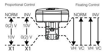
when the signal decreases. With the switch in the INV, the actuator spindle moves down when the signal decreases.
