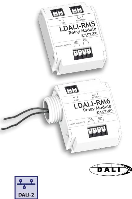
The LDALI-RM Relay Modules enable the control of consumers without DALI interface. Typical application scenarios are the integration of non-DALI luminaires (with 1 – 10V or no control interface) or other loads like fans in toilets or washrooms and motors for partition walls or screens in DALI lighting applications.
