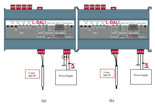
Figure 34: Connecting the LDALI-ME20X: (a) 2-wire MS/TP, (b) 3-wire MS/TP.
