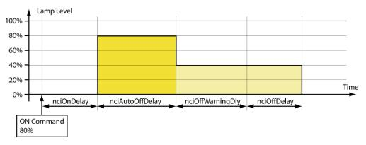
Figure 137: Timing Parameters with nciAutoOffDelay and nciOffWarningDly
