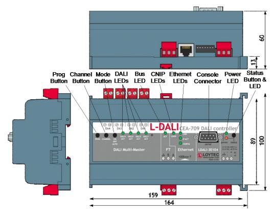
Figure 33: L-DALI Enclosure (dimensions in mm)
