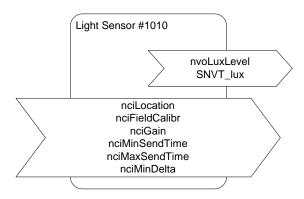
Figure 141: Light Sensor Object
