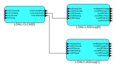
Figure 31: Network Variable Bindings
