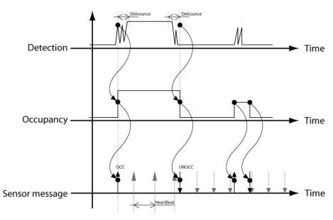
Figure 143: Timing of occupancy detection.
