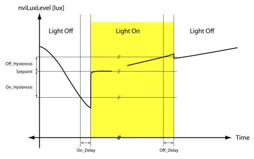
Figure 158: Constant Light Controller Timing.
