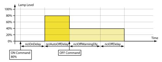
Figure 139: Timing Parameters (*nciAutoOffBreak*=ST\_ON)
