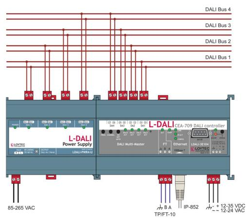
Figure 4: Basic Hardware Installation.
