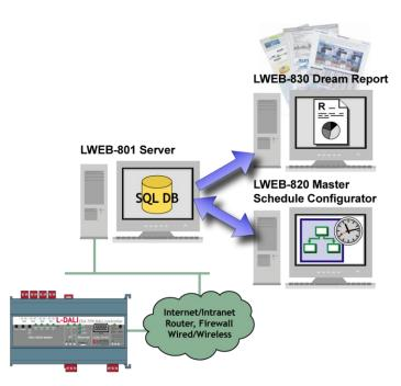
Figure 2: Using L-DALI together with the L-WEB product family
