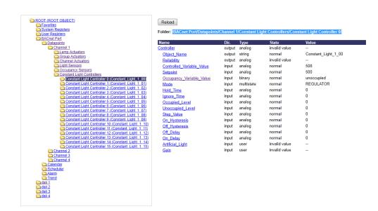
Figure 30 DALI Installation Web Interface: Parameters
