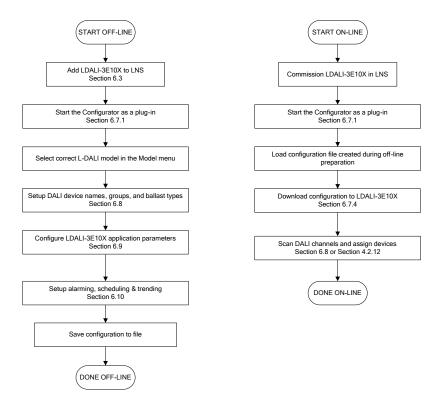
Figure 84: Basic off-line design-flow.
