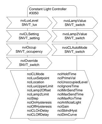
Figure 144: Constant Light Controller Object
