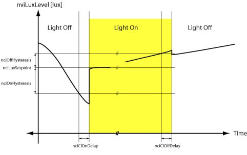
Figure 148: Constant Light Controller Timing
