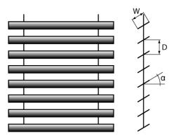
Figure 150: Sunblind Geometry
