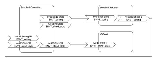
Figure 152: Controlling a Sunblind Actuator via SNVT\_setting
