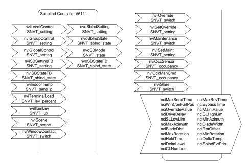
Figure 149: Sunblind Controller Object
