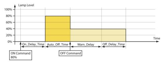
Figure 157: Timing Parameters (break enabled).
