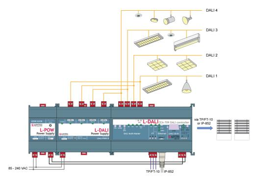
Figure 1: L-DALI supports up to four DALI channels
