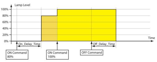
Figure 154: Timing Parameters.
