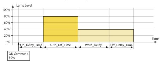
Figure 155: Timing Parameters with Auto\_Off\_Time and Warn\_Delay.
