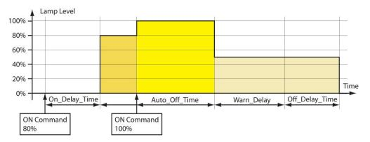
Figure 156: Timing Parameters (restart enabled).
