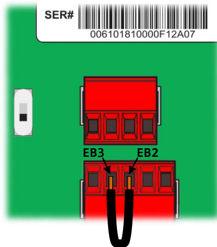
Figure 16: Cable Bridge EB2-EB3
