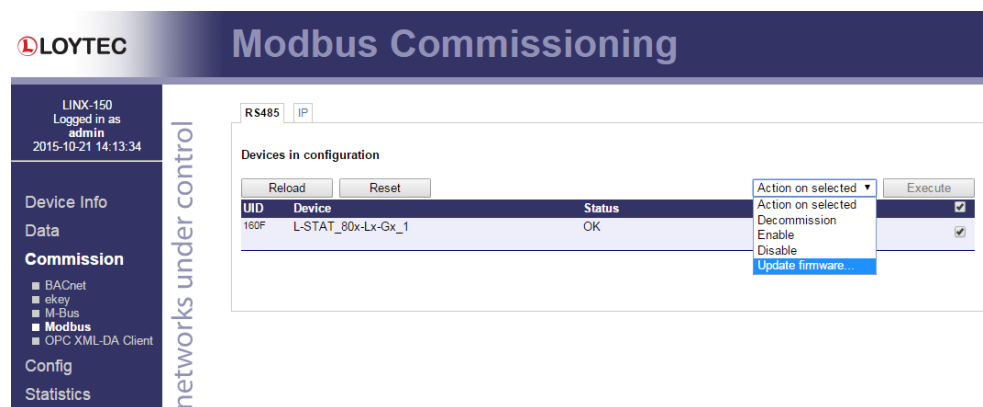
Figure 13: Web Interface – Modbus Commission
