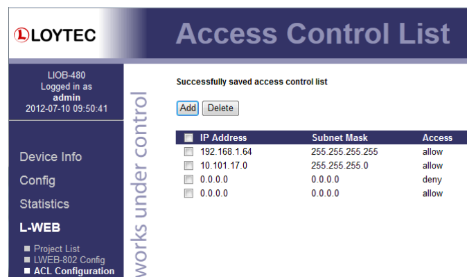
Figure 65: OPC Server Access Control List (ACL)
