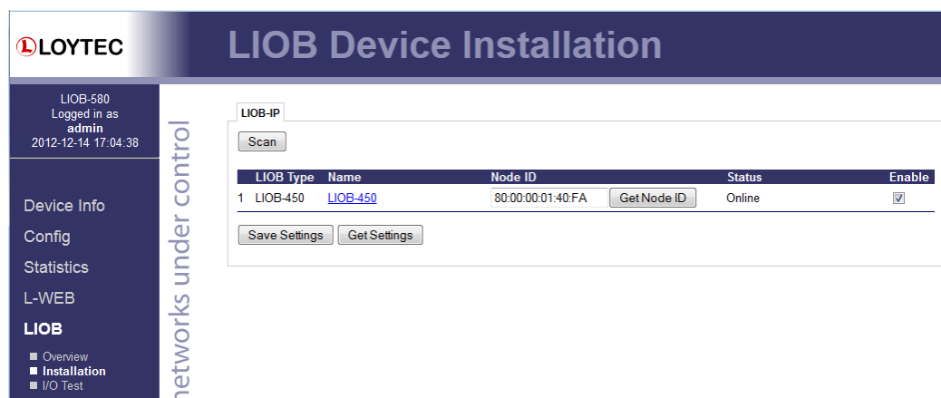
Figure 67: LIOB-IP Device Installation and Scan
