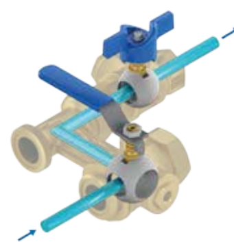
Forward flush from the return
