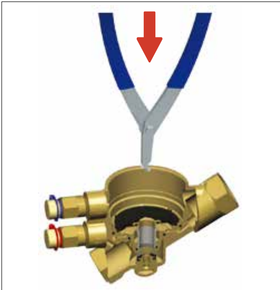
Step 5: Insert the nose pliers through the center of the cartridge
