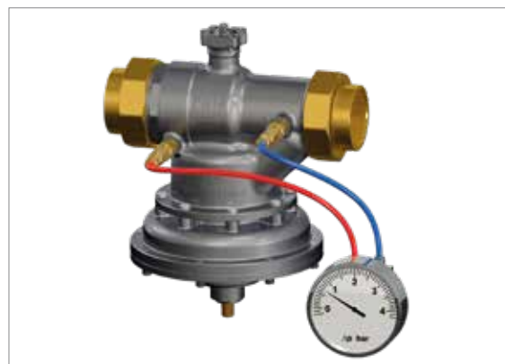
Lock again and re-open the valve. Don't overtighten. Could seriously damage the device. Torque 2÷3 Nm
