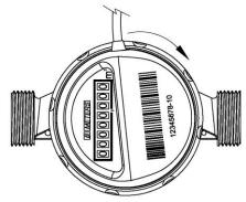
Turn clockwise the RFM-MB1 module until the module is blocked.
