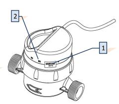
Two options are available to prevent the fraudulent module removal: 1.to stick a self destroying security label included in the package, between the meter capsule side edge and the module side edge.
