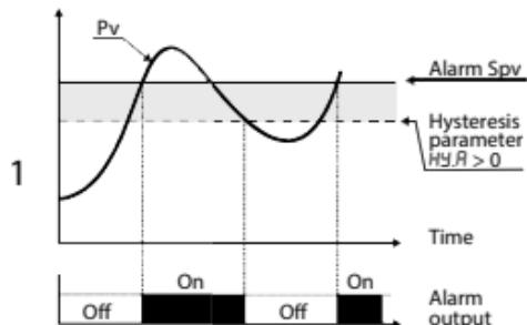
Absolute alarm with controller in heating functioning (par. 11  $rEG.$  come  $HEA | HEB$ ) and hysteresis (par. 23  $HY.R | HY5.R$ ) in absolute value.
