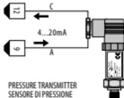
For signals 0/4...20mA with two-wire sensor
