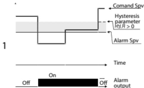
Absolute alarm refers to the command set, with the controller in heating functioning (par. 11  $r.EG.$  come  $HER | HER_E$ ) and hysteresis (par. 23  $HY.R | HY5.R$ ) in absolute value. The command set can be modified pressing the arrow keys or using the serial port RS485 commands. (only on ATR121/141-ADT).
