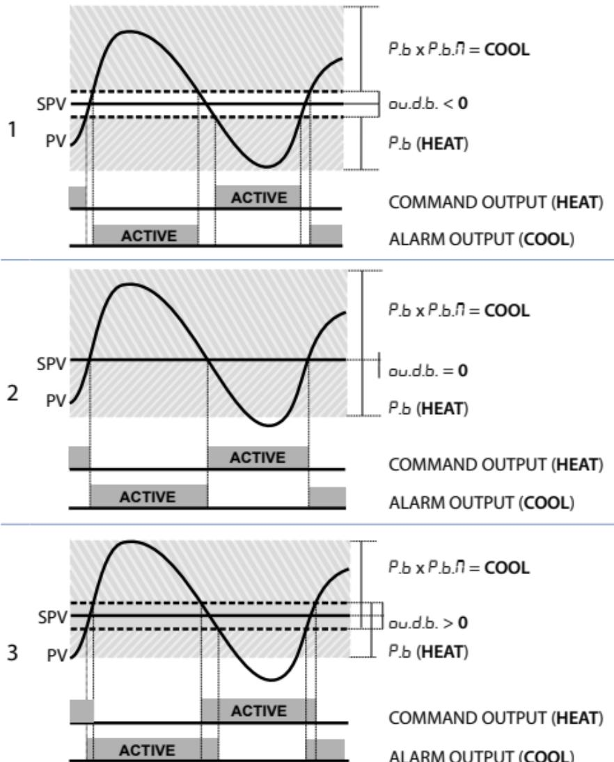
Parameter  $t.c.2$  has the same meaning of the cycle time  $t.c.$  for heating. Parameter  $co.F$  |  $coo.F$  (cooling fluid) pre-selects the proportional band multiplier  $P.b.\Pi$  and the cooling PID cycle time  $t.c.2$  basing on the type of cooling fluid:
