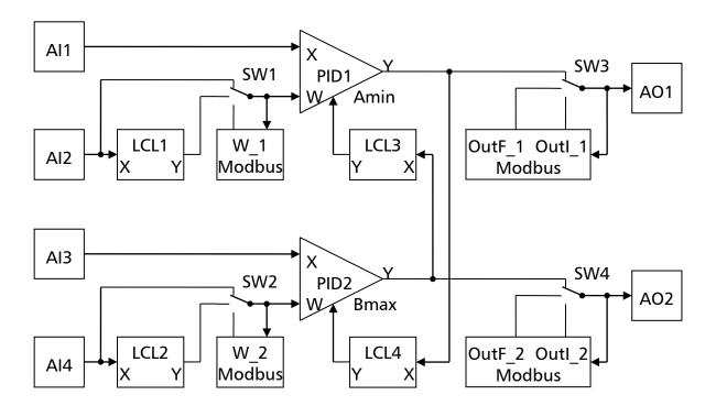
Depending on the operating mode, nominal value and actual value can originate from the analog inputs. These inputs provide values in Volts, Ohms or degrees of Celsius. If the function block Linear conversion / limit or freely programmable interpolation table is used in the analog input, adjustment to other value ranges and units can be performed at the controller input.
