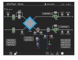
LWEB-803 is a graphical user interface to visualize dynamic pages showing plant details or a virtual room operator panel on a Microsoft Windows PC.
