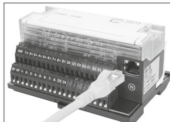
Connect the EWIO-9180 with a standard RJ45 patch cable to the Ethernet network.
